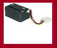
This allows writes to succeed according to the system, but actually blocks the interrupts from reaching the HDD
