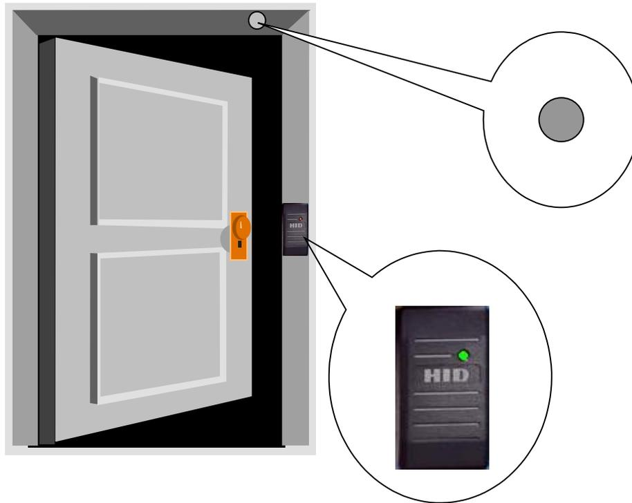
**In a system using proximity type cards, pass your access card (or similar credential) by the card reader. There are also various ways to allow exiting doors.**
